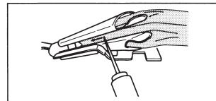
Use a long, narrow object to pull the bias tape through the inside of guide.
