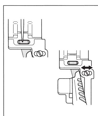
Place the cloth you wish to attach the bias tape to under the needle and align it with the center of the guide. Guide the cloth and bias tape so the tape does not extend over the edge of the fabric.
