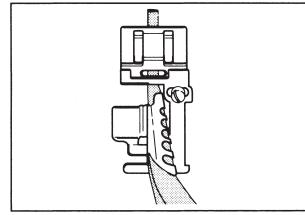
While making sure that both sides are folding inside the bias binder, pull tape slightly out behind foot (bias binder).
