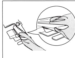
Feed bias tape (cut to 2.5cm) through grooves on front of guide of bias binder so that both sides of guide are lined up with both sides of tape.
