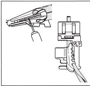
Use a long, narrow object to pull the bias tape through the inside of the guide. Pull tape out behind the rear of the foot.
