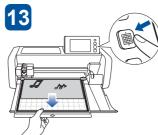
Press the "Feed" button in the operation panel to release the mat.
